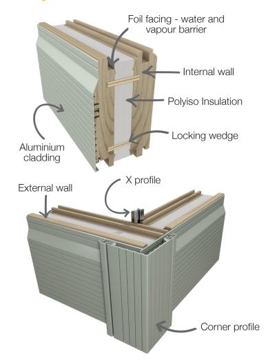
Polyisocyanurate, or Polyiso for short, is a thermoset insulation. This means that once it is cured it hardens and becomes permanently rigid.
